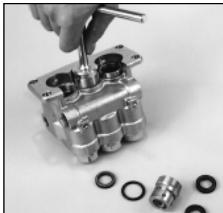
Removal of Seal Cases from Manifold Head
