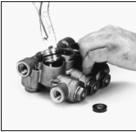
Removal of Seal Case and Lo-Pressure Seal
