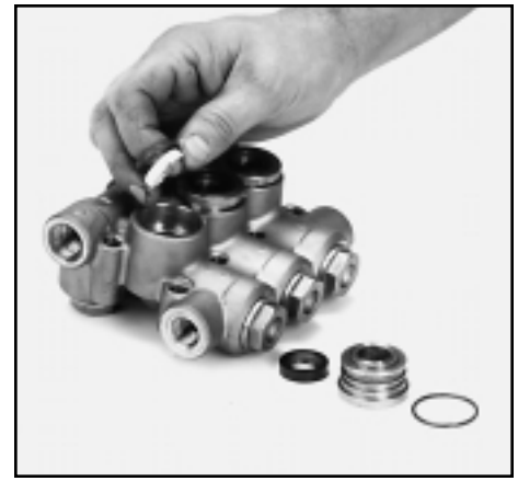
Reassembly of V-Packings
